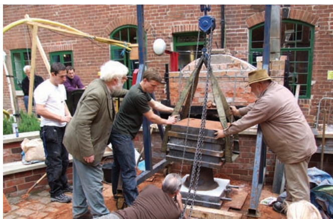
The box being carefully lowered over the mould.
