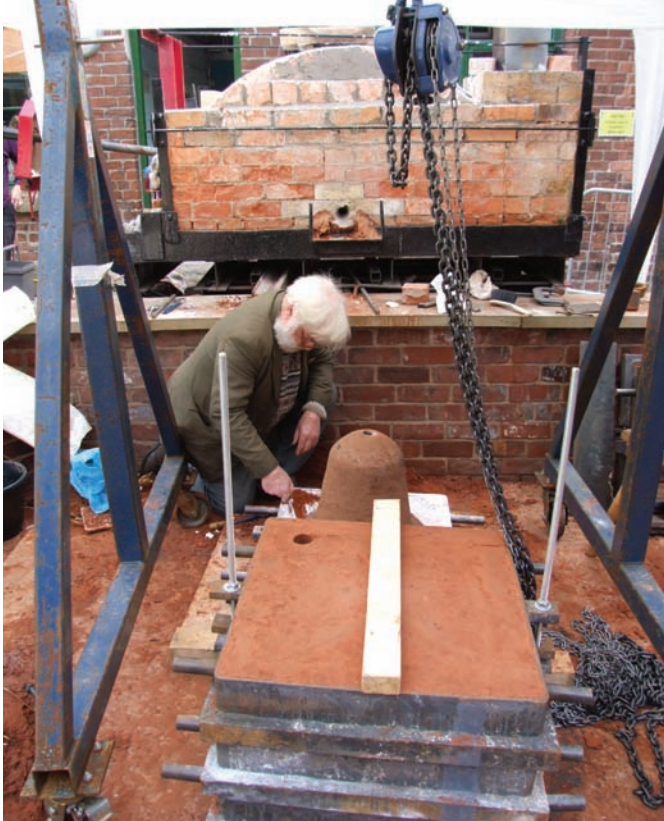
Bill making final preparations to the mould or cod
