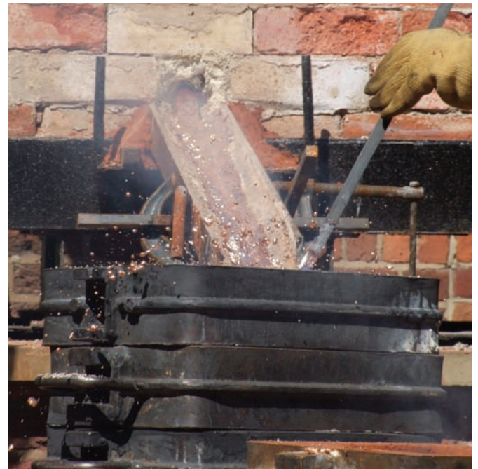
Boiling metal breaks loose into the slag pot
